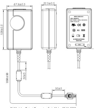
5V Models: Output Connector: 6 pin Molex 39-01-2060 or equiv. Pins 1, 4 = (+), pins 3, 6 = (-), pins 2, 5 = NC
